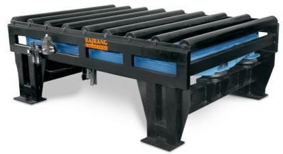
To ensure good molding results it is essential that the sand is well compacted and it is for this reason that "BAJRANG ENGINEERING" has taken particular care in the design and realization of the compaction tables. The most special feature is undoubtedly the possibility of regulating the frequency of the two electric vibrators, by means of a control inverter, positioned on the electrical panel itself.
