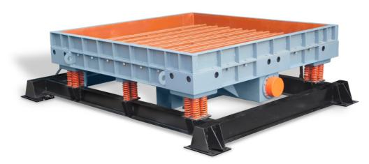
**BE SHAKEOUTS** are simple and robust machine designed for continuous duty to separate castings from sand, sand from flasks and cores from castings.
